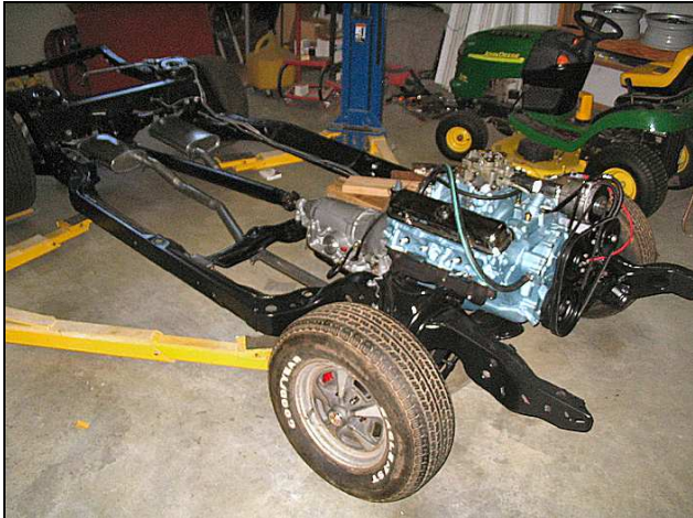
Project Update: Our 1969 GTO rebuilt engine and new overdrive transmission (2004R) are now back in the frame. Currently waiting for new radiator so that engine can be test fired up! It has been silent since 1989! Photo by Jon Stevens
